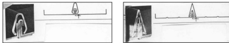
Figure 14.115-4: Low (3/8" x 1") and High (1/4" x 1-1/4") Roof Seams
