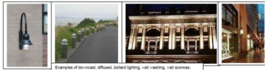
Figure 14.158-16: Downward and Diffused Lighting, Wall-Washing Lighting
