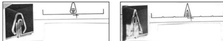
Figure 14.158-6: Low (3/8" x 1") and High (1/4" x 1-1/4") Roof Seams
