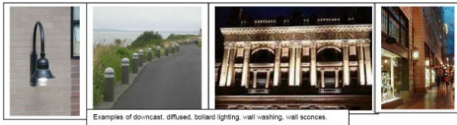
Figure 14.195-20: Downward and Diffused Lighting, Wall-Washing Lighting
